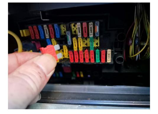
After pulling fuse 22 (7 along from the top left of the interior fusebox) the current draw went down to 10mA. 10mA is a very good number. There will always be a bit of draw - the BSI might only be half asleep, just waiting for someone to open a door, and there is a bit of electricity used to remember the time and settings. I'm very happy with 10mA.
