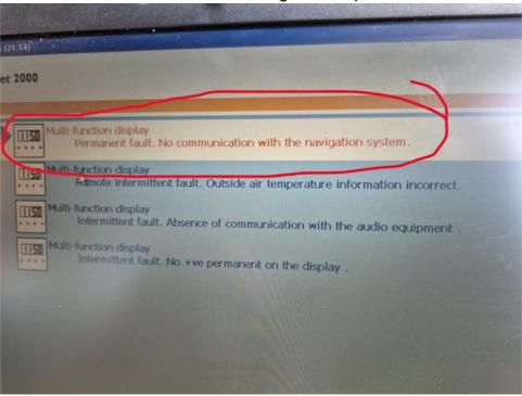
True enough the sat nav connector was a bit corroded. The CAN wires were probably dirty. I removed the sat nav ECU for weight saving and cable tied the connector off the floor to keep it dry.
