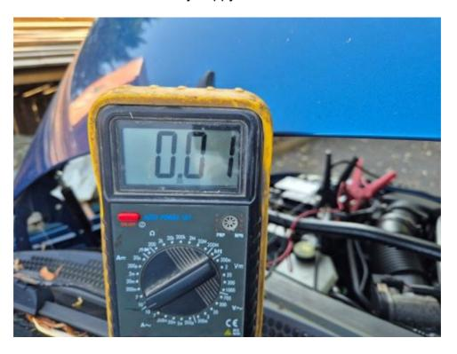
Fuse 22 is for interior courtesy lights and the rear view mirror. Removing the fuse reduced the draw by 40mA which works out at 0.5 watts. I'll check when it is dark whether there is some sun visor light staying on. Any tips about what else it might be appreciated of course.
